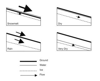
Figure 1. Water flows and relative position of the ice and water tables in a typical slope, under different meteorological conditions. The size of the arrows represents the difference in magnitude of the flow. The arrows above and inside the diagram represent the surface and the subsurface flow, respectively (redrawn from Woo 2000).
